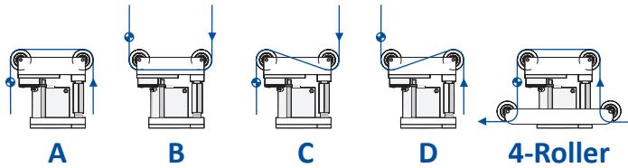
Guides can be placed in any orientation and sensor can be on either the near side or far side of the web. Dual sensor to center-guide is optional.
